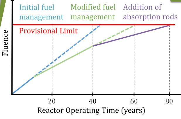
Why is fluence critical for nuclear reactor life extension? Fluence determines operational limits; managing flux can mitigate fluence accumulation, delaying the limit and extending RPV life.
